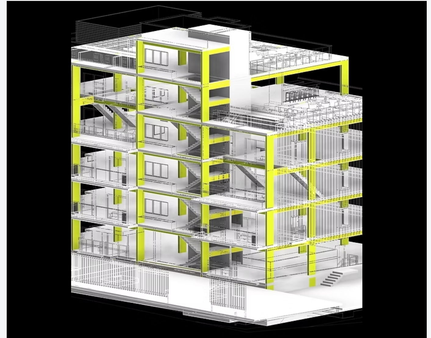
PATCADS STRUCTURAL MODEL
